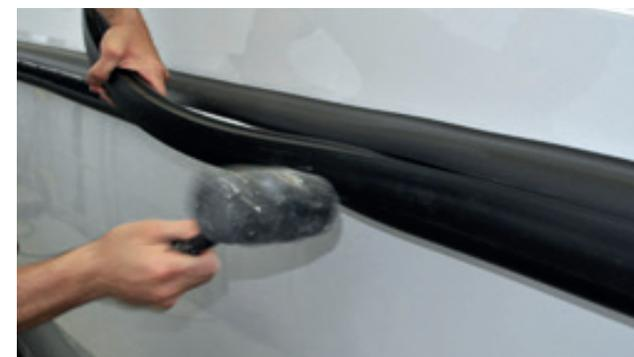
Install the top profile by pressing it with a rubber hammer.
