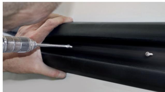
Drill and screw the base profile directly to the boat.
