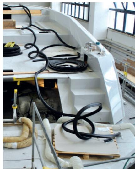
The Bino 40 profile consists of 2 modules, one base and one "top" which covers the fixing screws.
